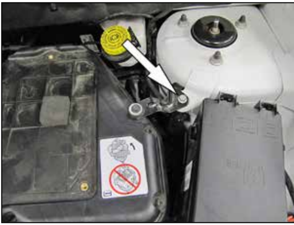
7. Remove the bolt securing the air box mounting bracket to the inner fender.
