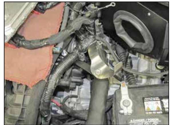
18. Unhook the wiring harness from the valve cover mounting stud, install the provided flat washer onto the stud and then install the tube mounting bracket assembly and secure with the provided washer and locking nut.
