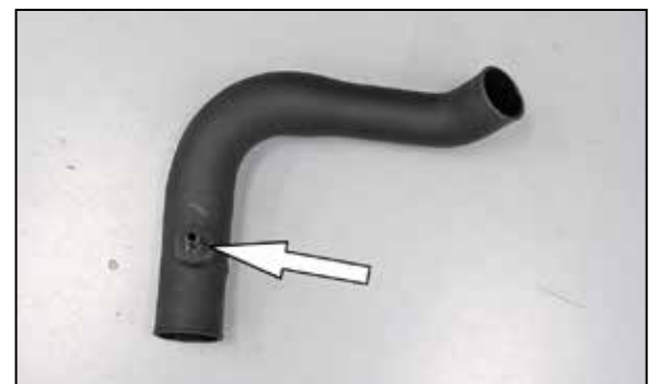
19. Install the provided vent fitting into the K&N® intake tube as shown. NOTE: Install the vent fitting "hand" tight, then turn it one complete turn with a wrench.
