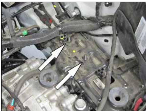
10. Unhook the wiring harness from the mounting studs.
