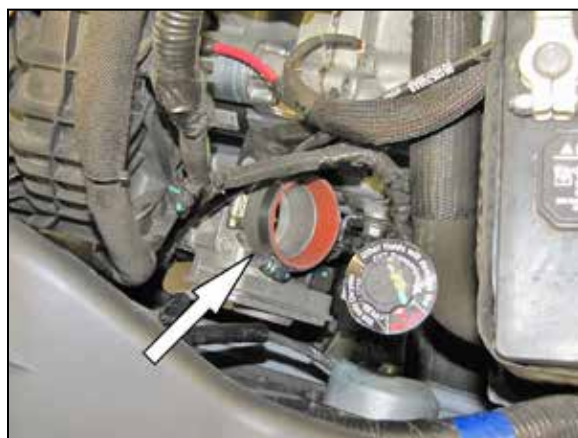
16. Install the provided silicone hose (08108) onto the throttle body and secure with the provided hose clamp.
