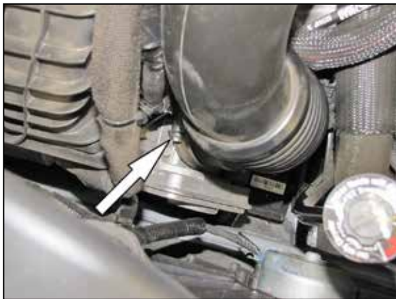
9. Loosen the hose clamp securing the stock intake tube to the throttle body and then remove the intake tube from the vehicle.
